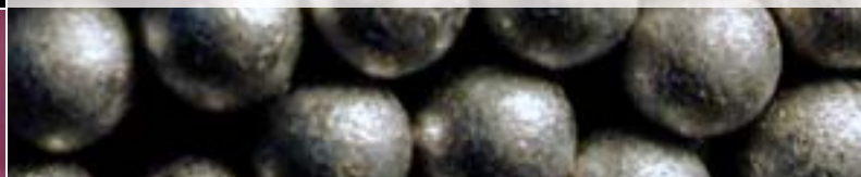
> Sample made up of aluminium beads 4.11 mm in diameter, used to study Anderson localization in three dimensions with acoustic waves.
