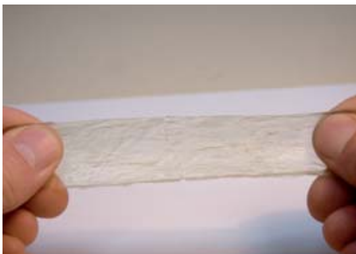
> This self-healing rubber can glue itself back together without being previously heated. Below, the rubber being tested by being pulled apart after self-healing.
